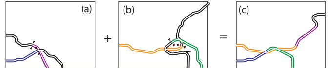
Fig. 3. Example of the original join crossover: in (c), the blue segment of (a) and the green segment of (b) have been joined, while the purple segment of (a) and the yellow segment of (b) have been joined.
